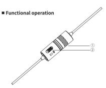
1) Battery compartment, loaded with LR44 battery
